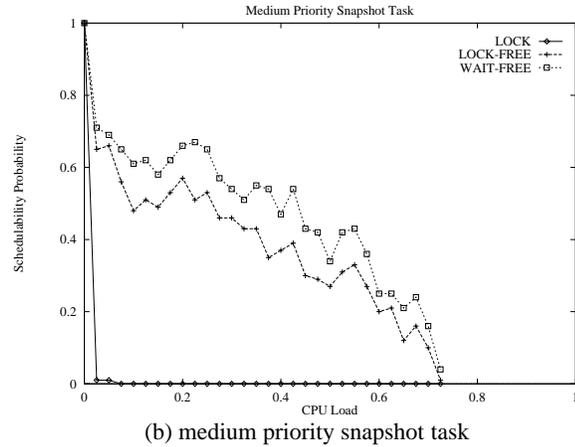
**Figure 5.** Schedulability admission tests for system with the parameters given in figure 6.
