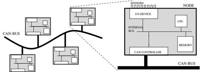
**Figure 7.** A CAN-based architecture with four micro-controllers
