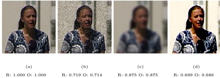
**Fig. 7.** The results of performing *SSIM* calculation using our optimized implementation (O) and the reference implementation (R) for an undistorted image (a), noisy image (b), blurred image (c), and an image with distorted levels (d).
