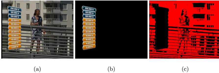
**Fig. 14.** Three images are produced when errors are detected, where (a) is the reference, (b) the actual output, and (c) the highlighted pixel error.
