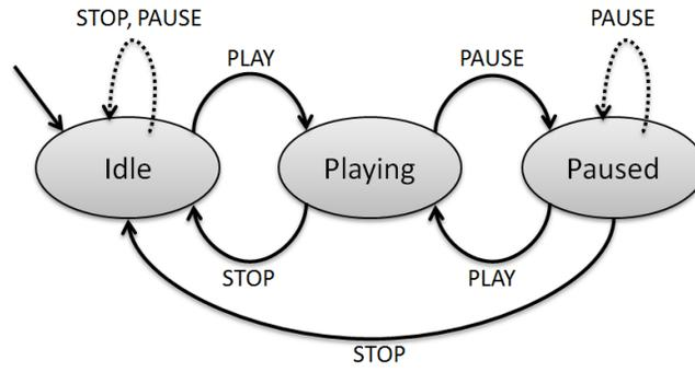
**Fig. 16.** A state machine showing parts of the formal definition used during the verification of *CasparCG*, where the invalid transitions detected are shown using dashed lines.
