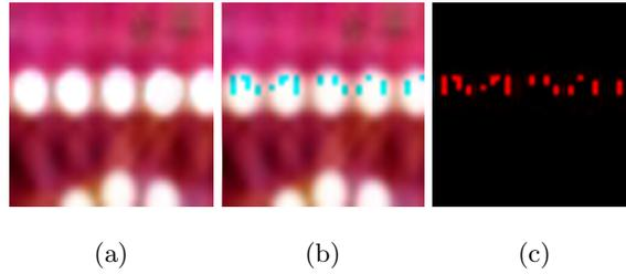
**Fig. 5.** Pixel rounding defect causing artifact to appear in image (b) which are not visible in the reference (a).
