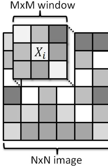
**Fig. 12.** The  $M$  by  $M$  window for the pixel  $X_i$  in the  $N$  by  $N$  image.
