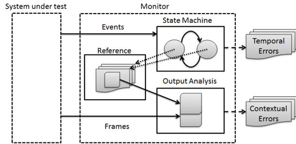
**Fig. 2.** The *RUGVEF* framework, used for automatically monitoring temporal and contextual properties of the system under test.
