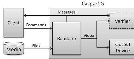
**Fig. 3.** The verifier is implemented as an input module, running as a part of *CasparCG*.
