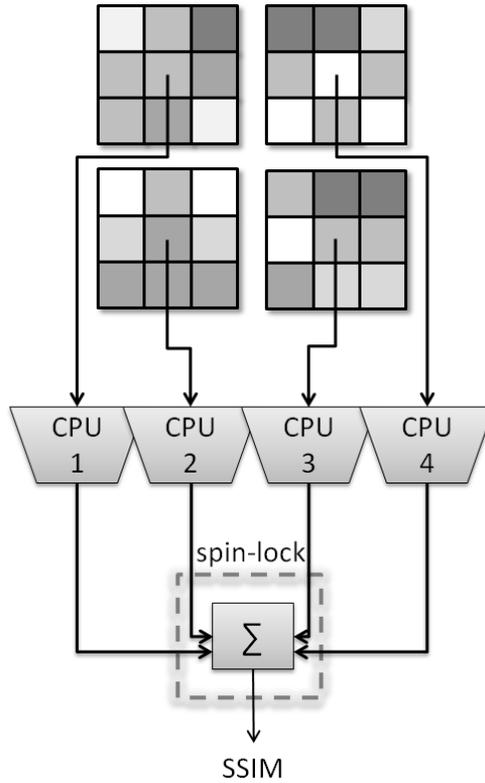
**Fig. 13.** Images are divided into partitions which are processed on different central processing units. The results of the partitions are then summed in a critical section using a low contention spinlock.
