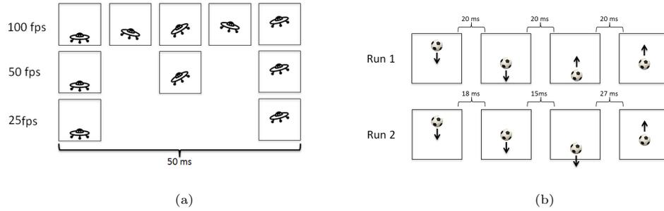
**Fig. 8.** (a) The frame-independent rendering technique renders a moving object at different frame rates, but where the displaced distance during identical periods is the same; (b) Frame-independent rendering produces different results depending on the time elapsed between each rendered frame.
