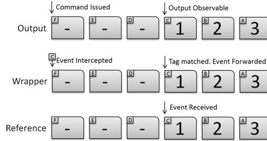
**Fig. 10.** Synchronization using a wrapper delays events until frames with correct tags are received.
