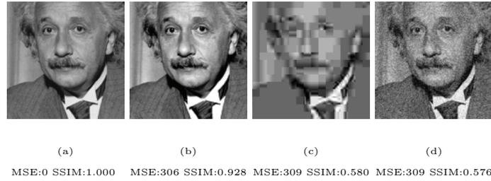
**Fig. 1.** *Image Quality Assessment* of distorted images using *MSE* and *SSIM* [16].
