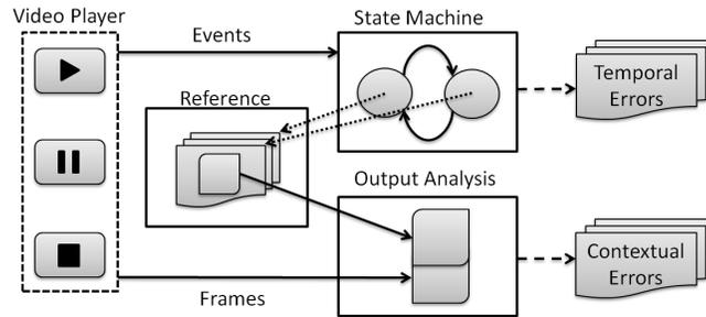
**Fig. 9.** An implementation of *RUGVEF* used for automatically monitoring the simple video player’s temporal and contextual properties.
