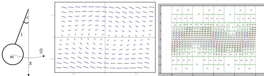
**Fig. 1.** On the left, the pendulum, with mass  $m$ , length  $l$ , gravitational acceleration  $g$ , angle  $\theta$ , and angular velocity  $\frac{d\theta}{dt}$ . In the middle, the phase plane of the pendulum, with  $m = 1, c = 2.5, l = 10, g = 10$ . On the right, a corresponding GSPDI
