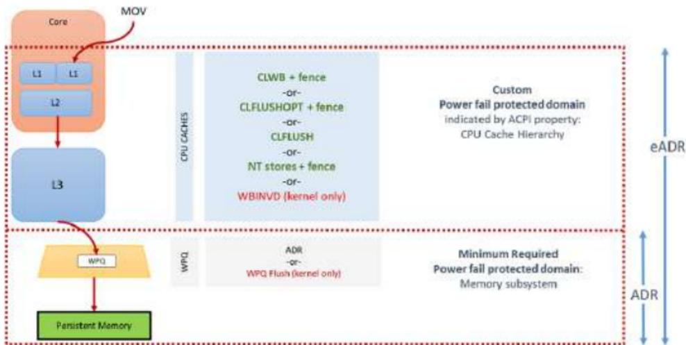
Figure: Power-fail protection domain on Intel platforms.
