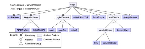
Fig. 4: Feature model of the TIAGo robot (excerpt). The model shows several features that a TIAGo robot may incorporate and the versions that can be equipped (e.g., different types of navigation lasers or RGBD cameras). The cross-tree constraints at the top-left indicate that the equippment of fingertip sensors require a specific parallel gripper and the force-torque sensor a robotic arm with seven degrees of freedom (DoF).
