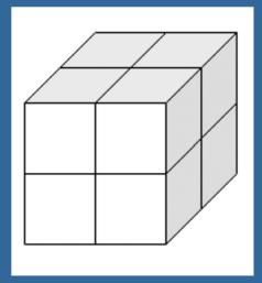
Recursively split space in eight parts – equaly along x,y,z dimension simultaneously for each level
