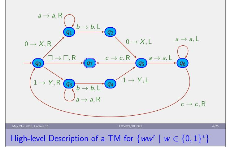
If in the initial state q₀ we read □, the word is empty so we move to q<sub>7</sub> and accept. Otherwise, if we read 0 (resp. 1) then we mark it with X (resp. Y), move R and change to the state q<sub>1</sub> (resp. q<sub>3</sub>) that will search for the corresponding 0 (resp. 1) at the end of the input.
