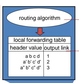
routing algorithm determines path through network (control-plane functionality)
