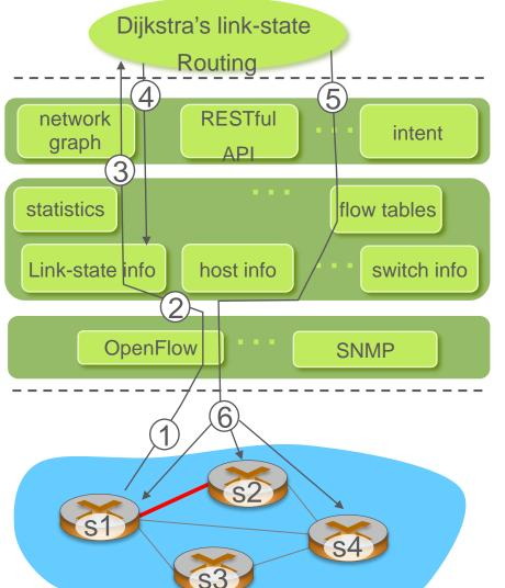
1) S1, experiencing link failure using OpenFlow port status message to notify controller
