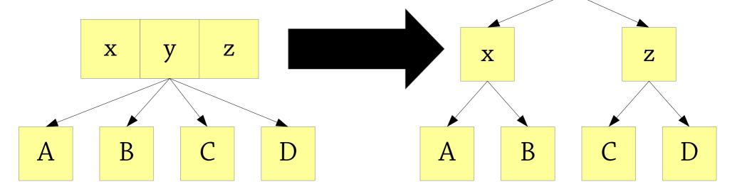
After splitting, we absorb the "extra level" node into its parent.
