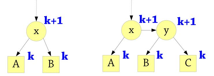
Notice that the level of x/y must be exactly one more than the level of A/B/C
