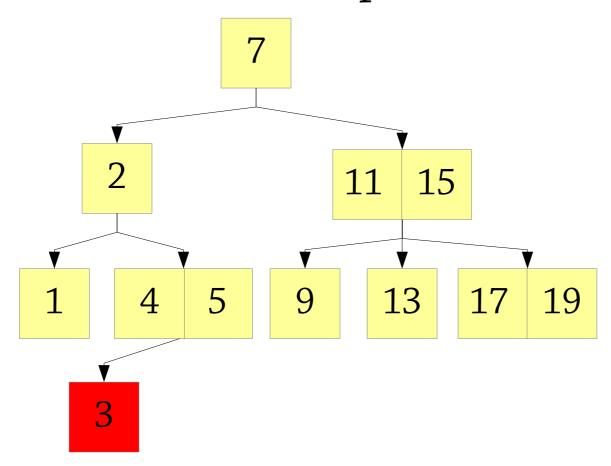
We get a 4-node, which is not allowed! We fix this by a method called *splitting*.
