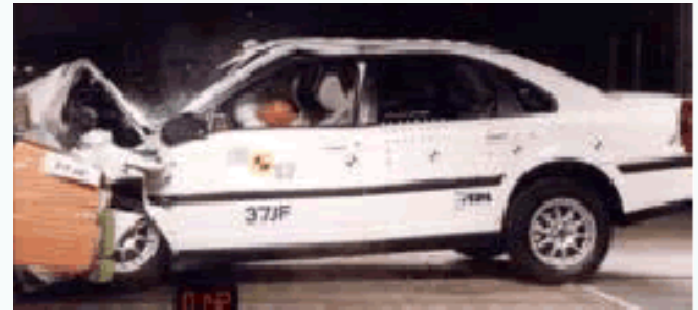
Offset crash test at 64km/h
