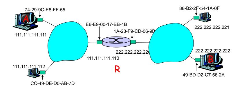
two ARP tables in router R, one for each IP network (LAN)
