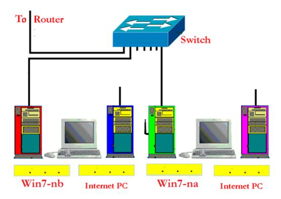
Exercise 1: Your computers are configured in a **Peer-to-peer LAN** connection. Find out what IP addresses the two Windows computers have by using, for example, the command **ipconfig /all** on the Command Prompt (you may need to run **cmd** first).
