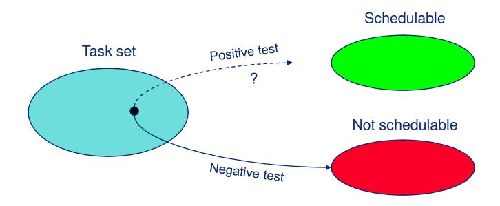
An <u>exact</u> feasibility test is both sufficient and necessary. If the answer is positive the task set is definitely schedulable, and if the answer is negative the task set is definitely not schedulable.
