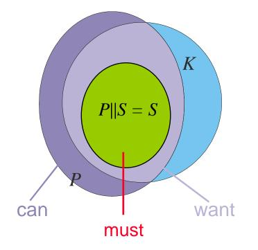
Algorithm 1. Calculate  $T_0 = P || K$ 2. Find un-controllable states  $S_0 = f(P, T_0)$ 3.  $S_{i+1} = SupNB(S_i)$ 4.  $S_{i+2} = SupC(S_{i+1})$ 5. If  $S_{i+2} \neq S_{i+1}$ , go to 3 6.  $S := S_{i+1}$
