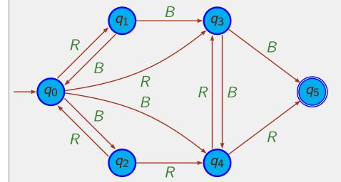
$q_0$  starts with B and R  $q_1$  both start with B  $q_2$  both start with R  $q_3$  starts with B and  $\epsilon$   $q_4$  starts with R and  $\epsilon$   $q_5$  both  $\epsilon$
