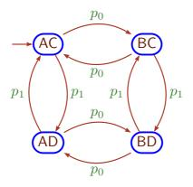
If after reading the word w we are in the state AD we know that w contains an even number of  $p_0$ 's and an odd number of  $p_1$ 's.
