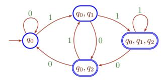
The DFA *remembers* the last two bits seen and accepts a word if the next-to-last bit is 1.
