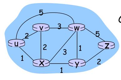
Clearly,  $d_v(z) = 5$ ,  $d_x(z) = 3$ ,  $d_w(z) = 3$ B-F equation says:  $d_u(z) = \min \{ c(u,v) + d_v(z), c(u,x) + d_x(z), c(u,w) + d_w(z), c(u,w) + d_w(z) \}$ = min {2 + 5, 1 + 3, 5 + 3} = 4
