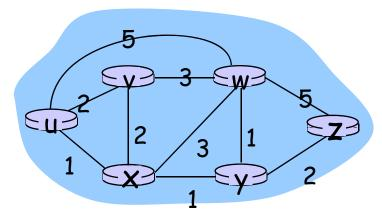
Graph: G = (N,E) N = set of routers = { u, v, w, x, y, z } E = set of links ={ (u,v), (u,x), (v,x), (v,w), (x,w), (x,y), (w,y), (w,z), (y,z) }
