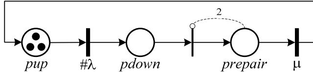
Markings of the GSPN model are represented as  $(\#pup \#pdown \#prepair)$ . The marking  $(0 \ 1 \ 2)$  corresponds to the event that the system is unavailable.
