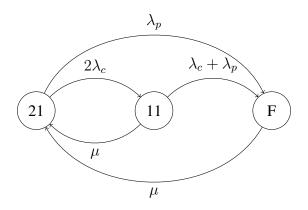
State label = # operational communication interfaces, # operational processors; F = failure.
