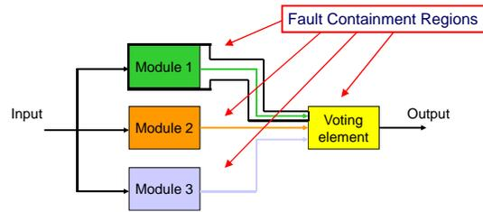
The designer must prevent that a fault in one module causes faults in the other module, or the voting element.
