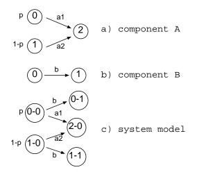
Figure 4.16: A Markov Model for a Series System
