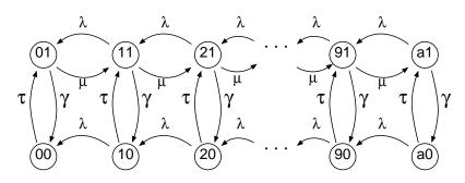
Figure 5.21: Markov Model for the Queueing System with Failure and Repair
