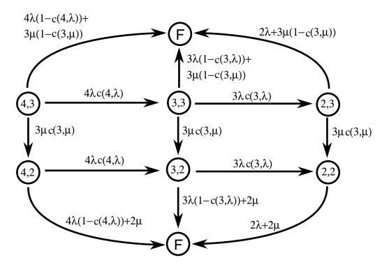
Figure 4.18: A Markov Model for a SIFT-like System
