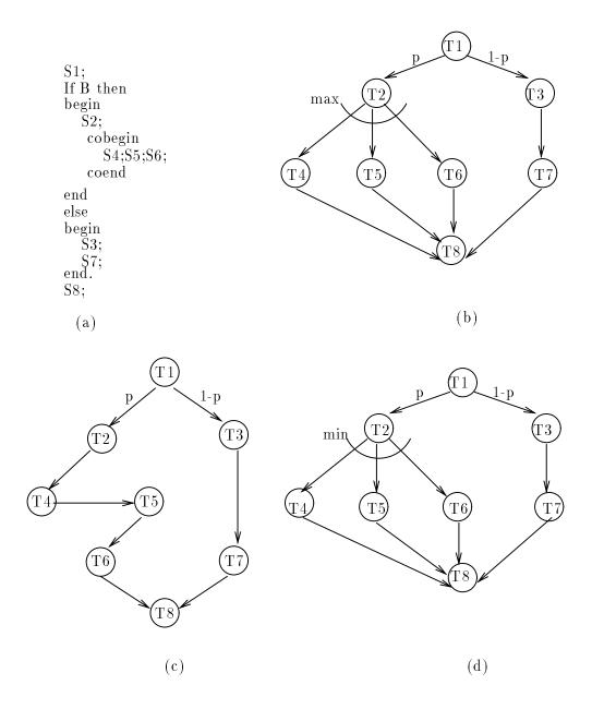
Figure 5.7: (a) Example parallel program. Graph models for the execution of the program on (b) 3 processors, (c) 1 processor, (d) "min" case
