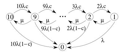
Figure 4.21: A Cyclic Markov Chain with Absorbing States
