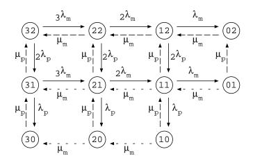
Figure 2.19: Markov chain model of 2-memory, 3-processor system
