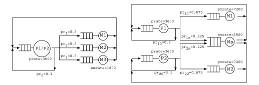
Figure 2.15: Queueing Network Models for the Two System Designs
