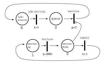
Figure 5.23: Petri Net Model for the Queueing System with Failure and Repair
