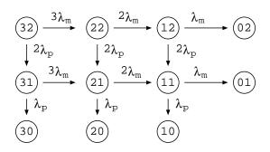
Figure 2.17: Markov Model of Shared-memory System
