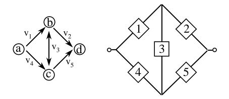
Figure 4.9: A Reliability Graph and Equivalent Non-series-parallel Block Diagram
