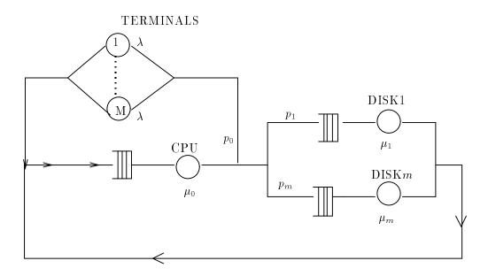
Figure 5.16: Terminal Oriented System
