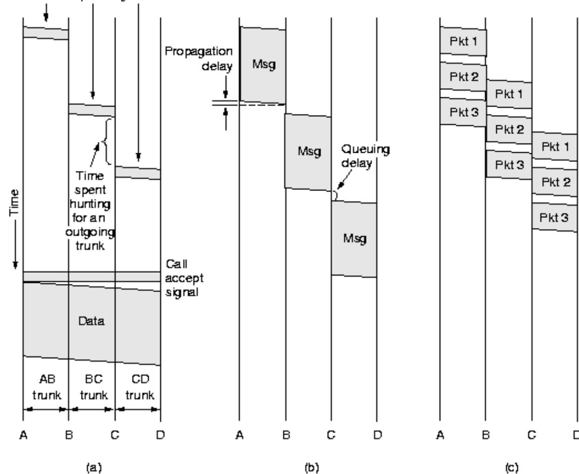
Fig. 2-35. Timing of events in (a) circuit switching, (b) message switching, (c) packet switching.
