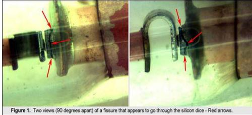
Figure 1. Two views (90 degrees apart) of a fissure that appears to go through the silicon dice - Red arrows.
