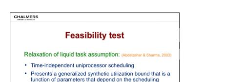
For deadline-monotonic scheduling, the synthetic utilization bound reduces to the optimal bound for liquid tasks
