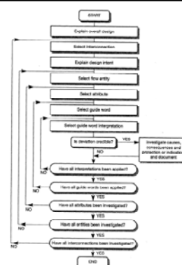
Figure 3.4 A flowchart of the HAZOP study process.
