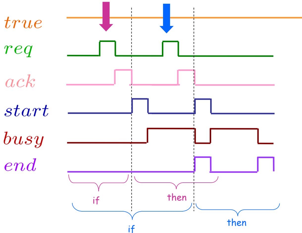
$\{\text{true}[*]; \text{req}; \text{ack}\} \Rightarrow \{\text{start}; \text{data}[*]; \text{end}\}$
