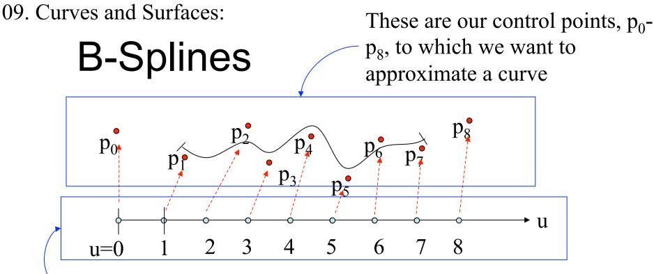
Illustration of how the control points are evenly (uniformly) distributed along the parameterisation u of the curve p(u).
