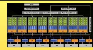
On NVIDIA 8000-series: Vertex-, Geometryand Fragment shaders allocated from a pool of 128 processors
