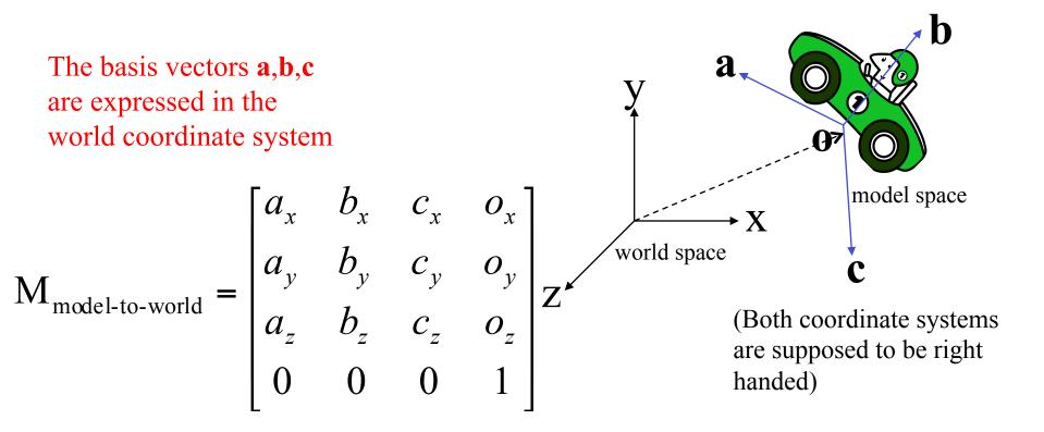
**E.g.:**  $\mathbf{p}_{\text{world}} = M_{\text{m}\to\text{w}} \mathbf{p}_{\text{model}} = M_{\text{m}\to\text{w}} (0,5,0)^{\text{T}} = 5 \mathbf{b} (+\mathbf{0})$
