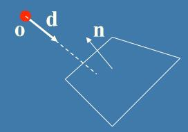
• Replace p by r(t) and solve for t:  $n \cdot (o+td) + d = 0$   $n \cdot o+tn \cdot d + d = 0$   $t = (-d - n \cdot o) / (n \cdot d)$ Here, one scalar equation and one unknown -> just solve for t.
