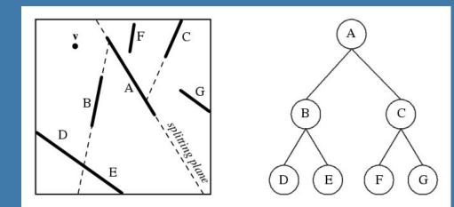
Know how to build it and how to traverse back-to-front or front-to-back with respect to the eye position (here: **v**)
