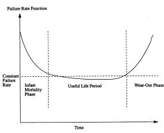
Figure 1.25: Illustration of the bathtub curve relationship. (From Barry W. Johnson, *Design and Analysis of Fault-Tolerant Digital Systems*, Addison-Wesley Publishing Company, Reading, Mass., 1989, p. 173.)
