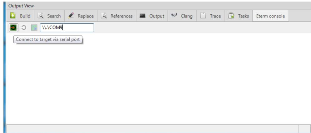
Click the leftmost button to connect to the MD407 card, and then press the red 'Reset' switch on the card to start its embedded monitor software. The "dbg:" prompt indicates that the monitor is ready to receive commands:
