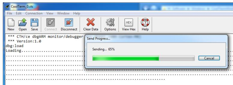
If the file transfer was successful your application program has been loaded into the RWM of the MD407 card, beginning at address 20000000<sub>16</sub>.
