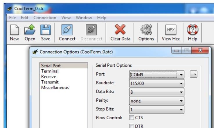
Click the 'Connect' button in CoolTerm to connect to the MD407 card, and then press the red 'Reset' switch on the card to start its embedded monitor software. The "dbg:" prompter indicates that the monitor is ready to receive commands:
