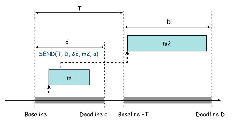
In this example, the SEND() moves the entire timing window of a method.
