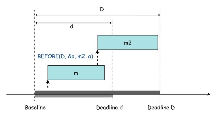
In this example, the BEFORE() call extends the timing window of a method.
