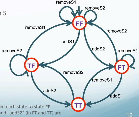
**Note:** Not included the "reset" action from each state to state FF Also, loops with "addS1" (in TF and TT), and "addS2" (in FT and TT) are missing (You could also have an implementation with no loops)
