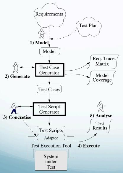
+ abstract tests + automatic execution + auto regression testing + auto design of tests + systematic coverage + measure coverage of model and requirements - modeling overhead Important: usually first abstract tests -> needs to get concrete tests: adaptor!
