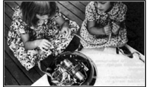
It can be directed by typing commands at the computer. The command `forward 100` causes the turtle to move forward in a straight line 100 "turtle steps". `right 45` rotates the turtle 45 degrees clockwise while leaving it in the same place on the floor. Then `forward 50` causes it to go forward 50 steps in the new direction.
