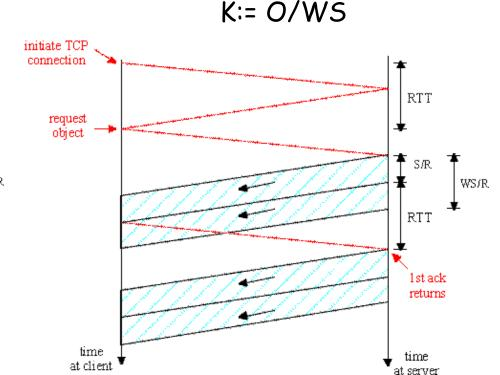
Case 2: WS/R < RTT + S/R: wait for ACK after sending window's worth of data sent delay = 2RTT + O/R + (K-1)[S/R + RTT - WS/R]
