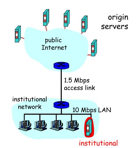
E(delay) = hitRatio\*LocalAccDelay + (1-hitRatio)\*RemoteAccDelay
