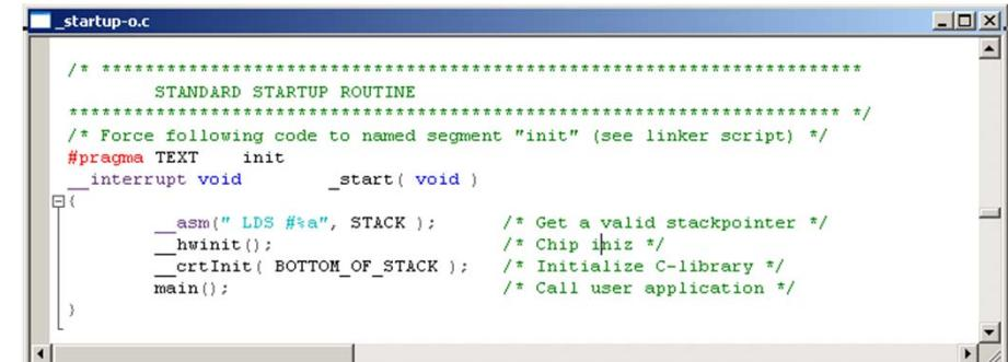
The screenshot shows a code editor window titled "startup-o.c". The code is a standard startup routine for a HCS12 microcontroller. It includes pragmas to force the code into the "init" segment and defines an interrupt handler for the application start. The code uses assembly-like syntax for stack initialization and calls to CRT initialization functions.
