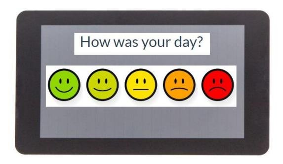
A touchscreen device presenting a web application. When an option is selected the application will send the data to a backend on Amazon Web Services. The data is saved in a database and visualized with QuickSight. The developed solution will be installed in the Cybercom office to test its performance and usefulness.
