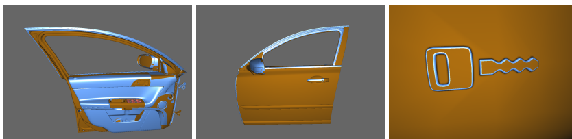
Figure 8: Before surface correction where blue/bright surfaces are front-facing (correct) and brown/dark surfaces are back-facing (incorrect).
