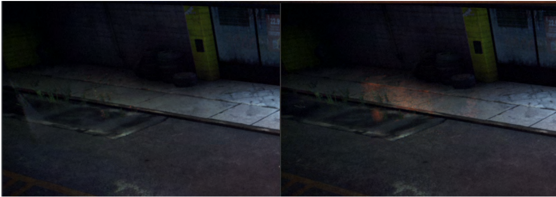
Figure 4.4: Unnatural emissive reflections when using IBL (right) compared to our method using ray tracing (left).
