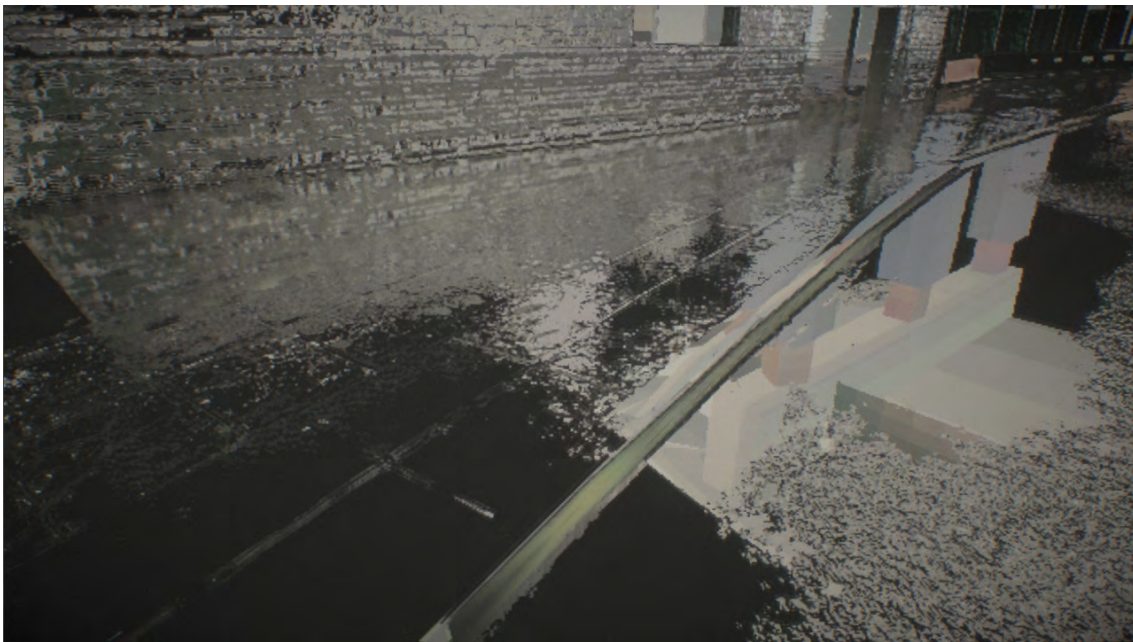
Figure 4.2: Mismatched proxy geometry, where the house does not exist in the generated proxy geometry. The texturing of the bridge pillars is also badly represented.
