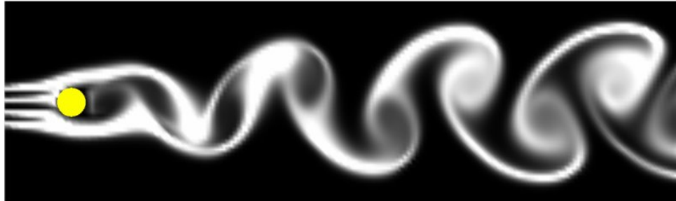
Figure 2.4: Picture from the work of Stam [41], showing the characteristic Von Karman vortex street produced behind an obstacle in a moving fluid.
