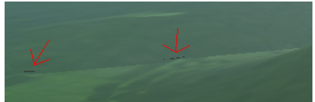
(b) Rendering of "cracks" artifact in a practical implementation of geomipmapping. Notice the holes, through which the gray background can be seen
