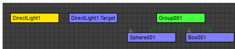
Figure 2 – A screenshot from 3ds Max 2012, showing parts of a scene graph where a sphere and a box is grouped together, and lit by a directional light with a target.
