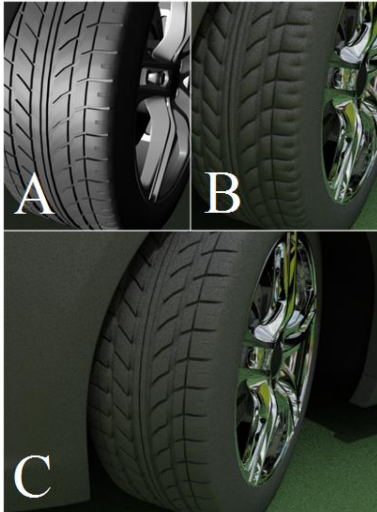
Figure 10 – Figure A shows a tire rendered with the default scanline renderer, figure B show the same tire rendered with the RapidRT plugin using normals from 3ds Max functionality, figure C shows our own implementation rendered with the RapidRT plugin, which is based on a solution suggested in 3ds Max SDK (Autodesk, 2011d).
