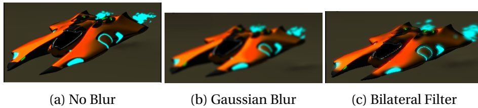
Figure 4.2.4: Comparison between different blur algorithms. In (b) using Gaussian Blur the whole image is blurred. With a Bilateral Filter (c) the edges are still sharp while the other parts of the image are blurred.
