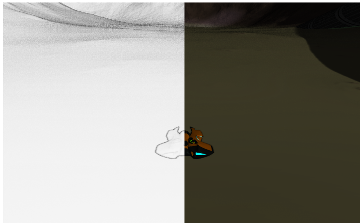
Figure 4.5.3: Comparison between ambient step(left) and final blend(right) without blur step. The noise of random sampling is clearly visible in the dark parts in the top of the image.
