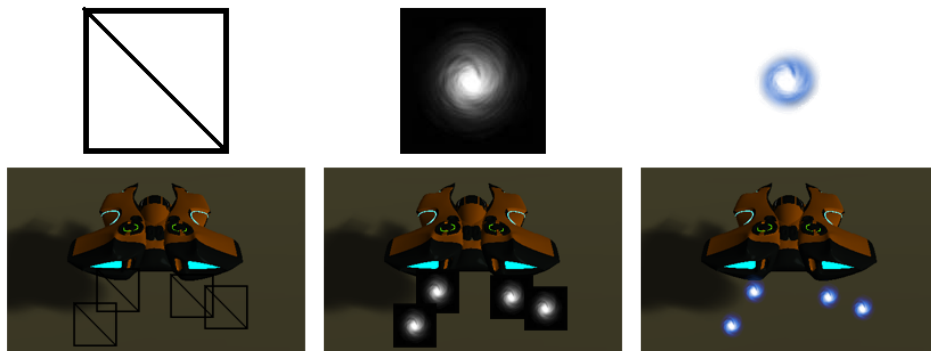
(a) The Particle as a 2D quad. (b) Texture applied to the quad. (c) Color and alpha added to the particle.
