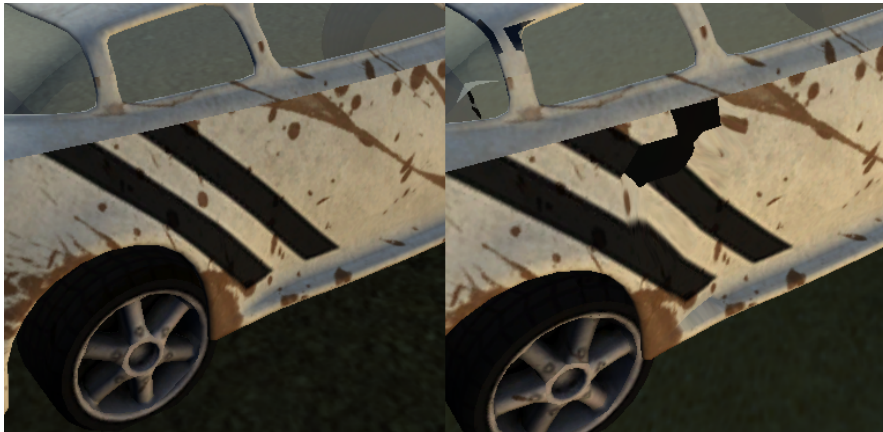
Figure 38: After a collision, vertex dislocation is applied to the unharmed vehicle (left), causing a dent, as seen in the striped area on the collided vehicle (right).
