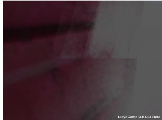
Figure 30: This is a comparison of a particle system in our game with and without soft particle rendering. The bottom half of this image uses soft particles, while the top half does not.
