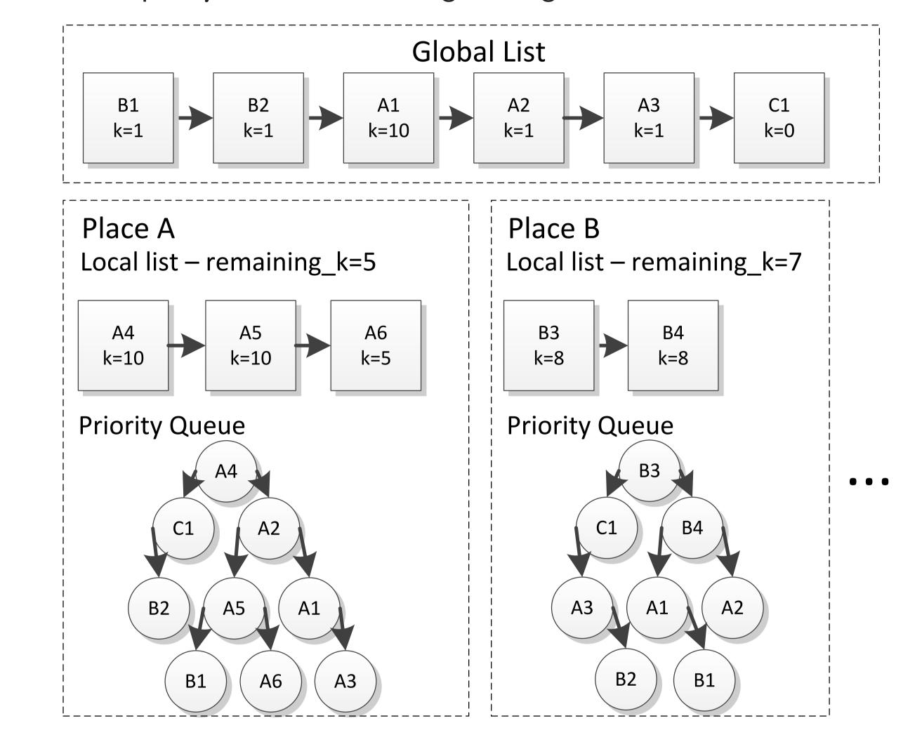
Each thread maintains its own list of tasks of length at most k. After ktasks were added to the list, the list is linked to a global list, thus making it public. Each thread maintains a serial priority queue with references to all tasks in the global list and its local list. If both lists are empty, a thread will spy tasks from another thread. Spying is similar to stealing in work-stealing systems, with the main difference being that the original owner still has access to a spied task.
