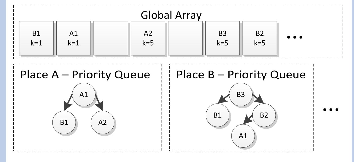
**Implementation:** Tasks stored in global array in order of creation, but may be shifted by up to k positions to reduce congestion. Priorities maintained locally using a serial priority queue per thread storing references to the global array. Each thread is allowed to ignore the latest  $m{k}$  tasks in the global array created by other threads.
