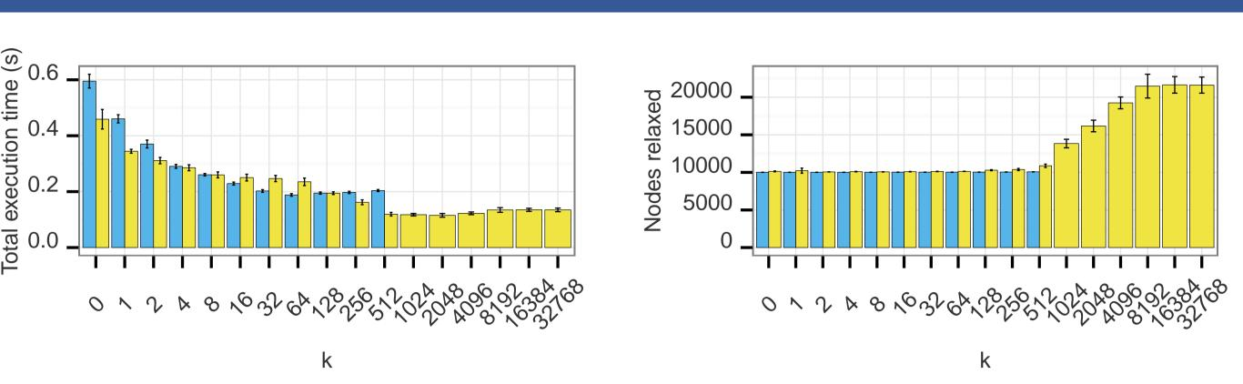
High overhead with small k, but close to optimal useless work with k up to 512. Best compromise between scalability and priority guarantees at k=512 in this case. (Intel Xeon E7-8850, n=10000, p=50%)
