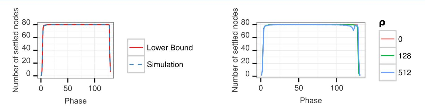
A simulation based on our theoretical model confirms the obtained upper bounds on useless work. Throughout most of the execution the expected useless work is very small. (n=10000, P=80, p=50%)
