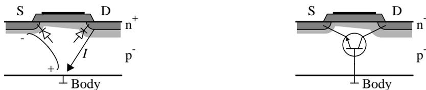
Fig. 31: Parasitic bipolar action in an n-type MOS.
