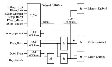
Fig. 2. Simplified Safety Code of Use Case Plant
