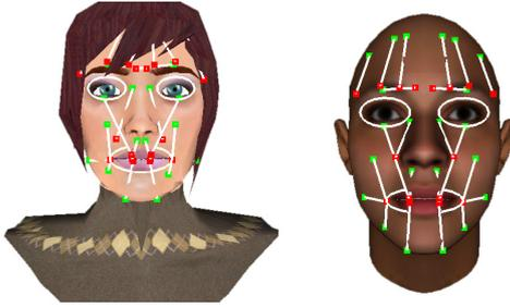
Figure 5: The resulting muscle map applied to different face meshes.
