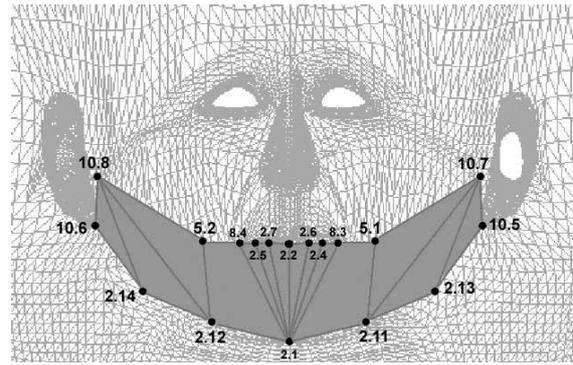
Figure 6: Cylindrical projection of the estimated jaw mesh through the use of some of the MPEG-4 FDPs.
